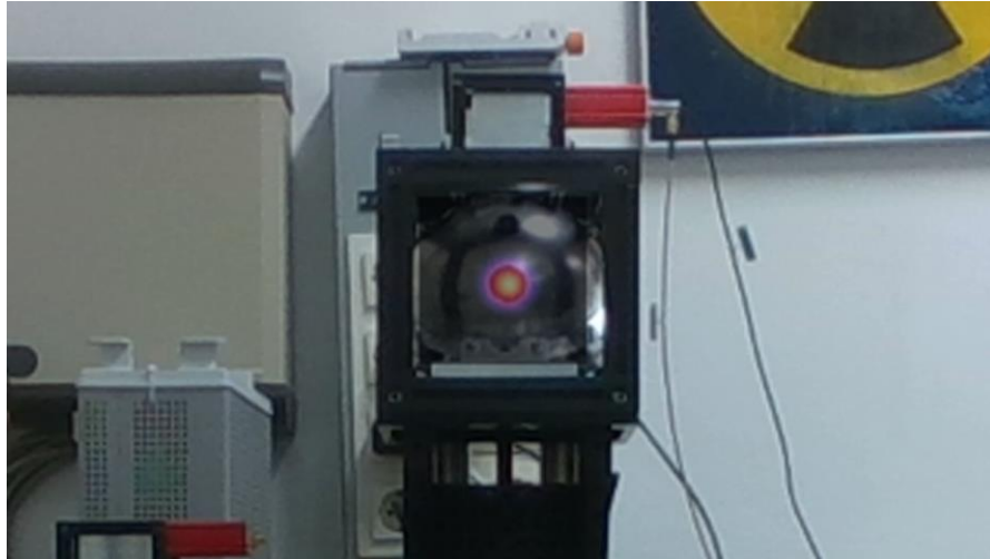
340 nm Radiance Standard Calibration against Po-210 Source
