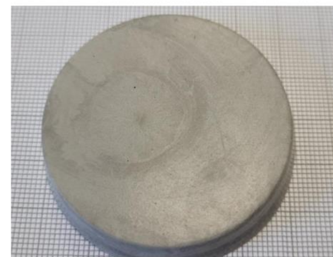
Concrete poured with an Am-241 solution (A. Klose, C. Walther | LUH)
