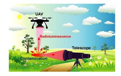
Use of air as a scintillator: radioluminescence (UV light, 200–440 nm)
