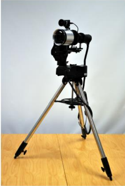
Radioluminescence mapping system based on a Galilean telescope built at Tampere University of Technology, Finland.
